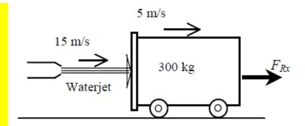
**Analysis** The braking force was determined in previous problem to be 250 N. When the brakes fail, this force will propel the cart forward, and the accelerating will be
