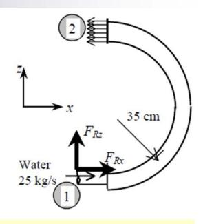
**Assumptions 1** The flow is steady, frictionless, one-dimensional, incompressible, and irrotational (so that the Bernoulli equation is applicable). **2** The weight of the elbow and the water in it is negligible. **3** The water is discharged to the atmosphere, and thus the gage pressure at the outlet is zero. **4** The momentum-flux correction factor for each inlet and outlet is given to be  $\beta = 1.03$ . **Properties** We take the density of water to be  $1000 \text{ kg/m}^3$ .
