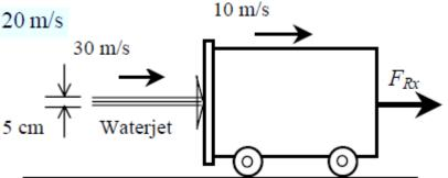
$\sum \vec{F} = \sum_{out} \beta \dot{m} \vec{V} - \sum_{in} \beta \dot{m} \vec{V}$ . We let the horizontal reaction force applied to the plate in the negative x direction to counteract the impulse of the water jet be  $F_{Rx}$ . Then the momentum equation along the x direction gives
