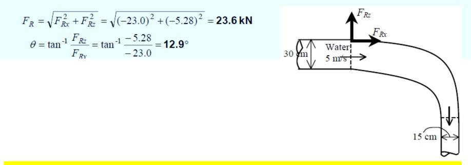
**Discussion** The magnitude of the anchoring force is 23.6 kN, and its line of action makes 12.9° from +x direction. Negative values for  $F_{Rx}$  and  $F_{Ry}$  indicate that the assumed directions are wrong, and should be reversed.
