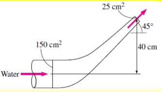
**Assumptions 1** The flow is steady, frictionless, one-dimensional, incompressible, and irrotational (so that the Bernoulli equation is applicable). **2** The weight of the elbow and the water in it is considered. **3** The water is discharged to the atmosphere, and thus the gage pressure at the outlet is zero. **4** The momentum-flux correction factor for each inlet and outlet is given to be  $\beta = 1.03$ .
