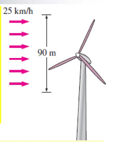
**Properties** The density of air is given to be 1.25 kg/m<sup>3</sup>. **Analysis** (a) The power potential of the wind is its kinetic energy, which is  $\dot{m}V^2/2$  per unit mass, and for a given mass flow rate:
