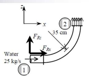
**Assumptions 1** The flow is steady, frictionless, incompressible, and irrotational (so that the Bernoulli equation is applicable). **2** The weight of the elbow and the water in it is negligible. **3** The water is discharged to the atmosphere, and thus the gage pressure at the outlet is zero. **4** The momentum-flux correction factor for each inlet and outlet is given to be  $\beta = 1.03$ .
