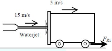
$$\sum \vec{F} = \sum_{\text{out}} \beta i n \vec{V} - \sum_{\text{in}} \beta i n \vec{V} \quad \rightarrow \quad F_{Rx} = -i n_i V_i \quad \rightarrow \quad F_{\text{brake}} = -i n V_r$$
