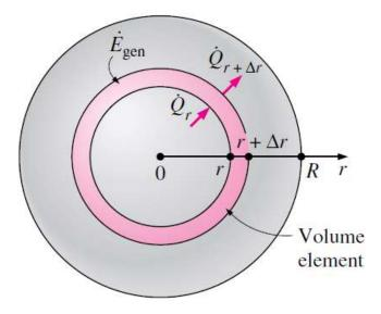
Variable conductivity  $\frac{1}{r^2} \frac{\partial}{\partial r} \left( r^2 k \frac{\partial T}{\partial r} \right) + \dot{e}_{gen} = \rho c \frac{\partial T}{\partial t}$ Constant conductivity  $\frac{1}{r^2} \frac{\partial}{\partial r} \left( r^2 \frac{\partial T}{\partial r} \right) + \frac{\dot{e}_{gen}}{k} = \frac{1}{\alpha} \frac{\partial T}{\partial t}$
