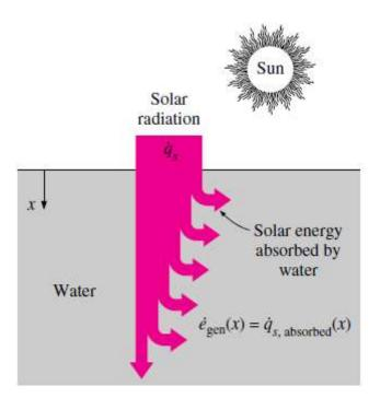
The absorption of solar radiation by water can be treated as heat generation.
