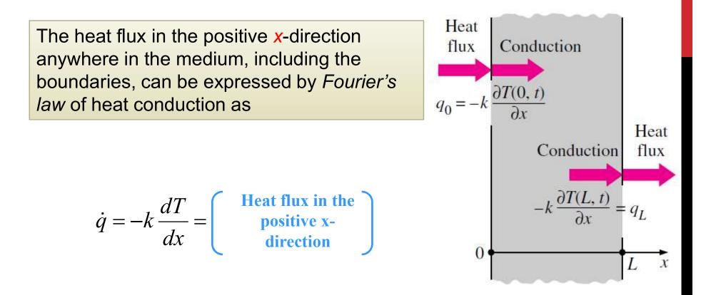
The sign of the specified heat flux is determined by inspection: *positive* if the heat flux is in the positive direction of the coordinate axis, and *negative* if it is in the opposite direction.
