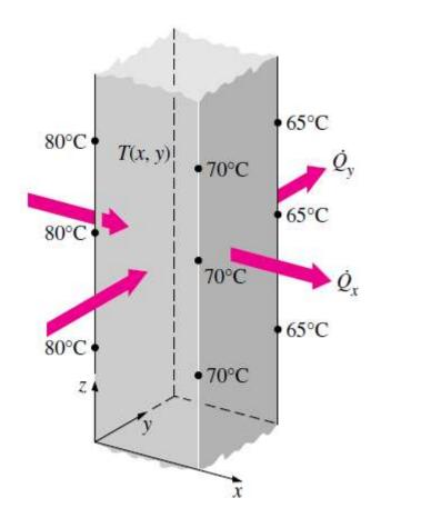
Two-dimensional heat transfer in a long rectangular bar.
