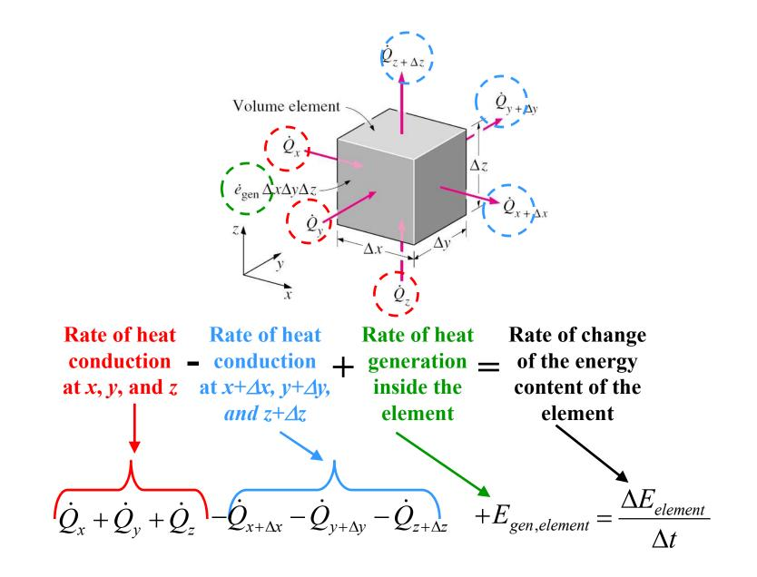
Repeating the mathematical approach used for the one-dimensional heat conduction the three-dimensional heat conduction equation is determined to be
