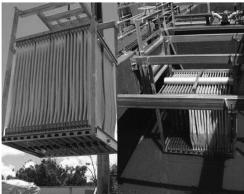
Figure 3.32 Schematic of the submerged membrane cassettes and the aerators.
