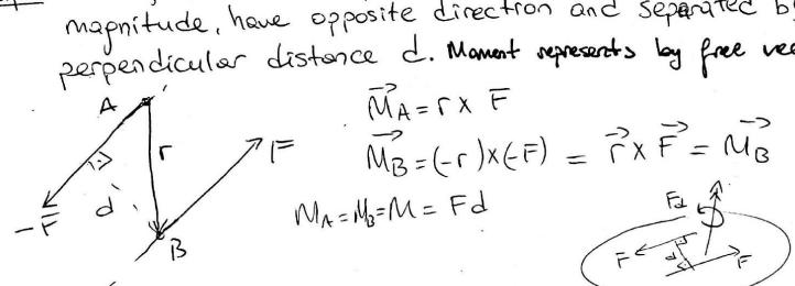
Equivalent Couple's Took Two Couples are said to be equivalent if they produce some moment. F=50 EN 2=2m > F= -50 EN 120 = Fz M = 2.50 = 100 kHM = 20,5 = 100 EN Moving a Force to a point out of its line of action No =7 X F Forces withsome magnitude but opposite sense Force Couple system one odded
