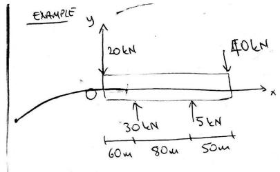
Find the resultant Force of piven Parellel forces applied on the ripid body?
