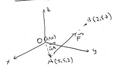
The force F is acting on the direction AB and its magnitude is F=10 kM. Move F? to point O.
