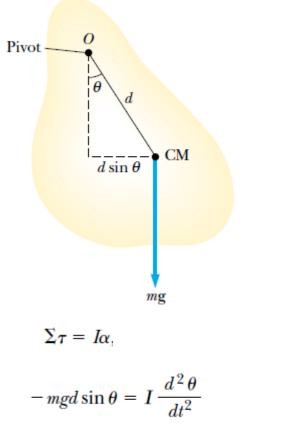
$\frac{d^2\theta}{dt^2} = -\left(\frac{mgd}{I}\right)\theta = -\omega^2\theta$  $\omega = \sqrt{\frac{mgd}{I}}$
