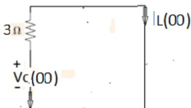
$$2. \text{durum} \quad I_L(\infty) = 0 = I_{Lzor} \quad V_C(\infty) = 0 = V_{Czor}$$
