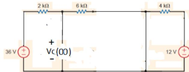
$$2. \text{ durum} \quad V_c(\infty) = \frac{36}{(2000+6000)}x 6000 = 27V = V_{czor} \quad \underline{5 \text{ puan}}$$
