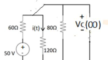
$$2.\text{durum} \quad V_c(\infty) = \frac{50}{\frac{120 \times 80}{120+80} + 60} \times \frac{120}{120+80} \times 80 = 22,222V = V_c \text{zor} \quad \underline{5 \text{ puan}}$$
