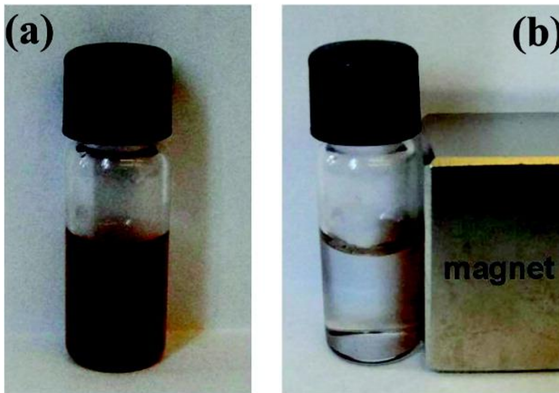
Images of PQA-modified nanoparticles (Table 1, entry 3) in water (2 mg/mL) (a) prior to and (b) after exposure to a permanent magnet for 10 min.
