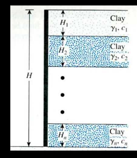
Sometimes, layers of both sand and clay are encountered when a braced cut is being constructed. In this case, Peck (1943) proposed that an equivalent value of cohesion should be determined according to the formula
