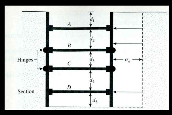
Step 2.Determine the reactions (A,B1,B2,C1,C2,D) for the two simple cantilever beams (top and bottom) and all the simple beams between.
