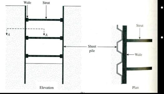
Construction of braced cuts using interlocking sheet pile;
