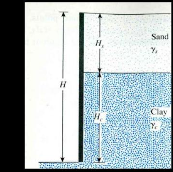
Once the average values of cohesion and unit weight are determined, the pressure envelopes in clay can be used to design the cuts.
