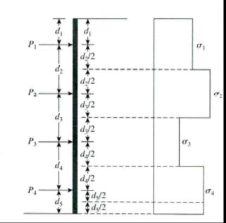
Using the procedure just described for strut loads observed from the Berlin subway cut, Munich subway cut, and New York subway cut, Peck (1969) provided the envelope of apparent-lateral-pressure diagrams for design of cuts in sand.
