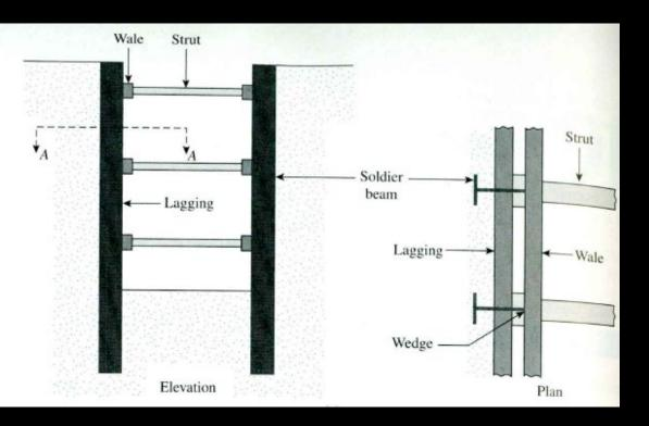
Construction of braced cuts using soldier beam;
