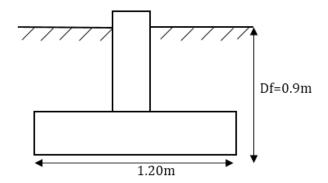
A strip foundation is shown in figure. The soil supporting the foundation has a friction angle of  $20^{\circ}$  and c'=20 kN/m<sup>2</sup>. The unit weight of soil, is 17.30 kN/m<sup>3</sup>.
