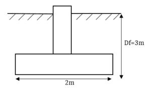
A strip foundation with 2m width is shown in the figure. The soil supporting the foundation has a friction angle of  $15^{\circ}$  and c=7 t/m $^{2}$ . The saturated unit weight of the soil is 2.0 t/m $^{2}$  and natural unit weight of the soil, is 1.71 t/m $^{2}$ .
