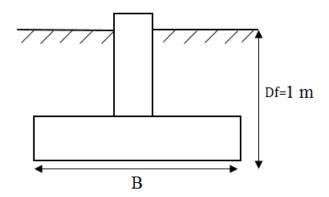
For the square foundation shown in the figure , the gross allowable load,  $Q_{all}$ , with FS=3 is 294.3 kN. If the supporting sandy soil has a friction angle of  $35^{\circ}$ and unit weight of  $18.15 \text{ kN/m}^3$ , determine the size of the footing.
