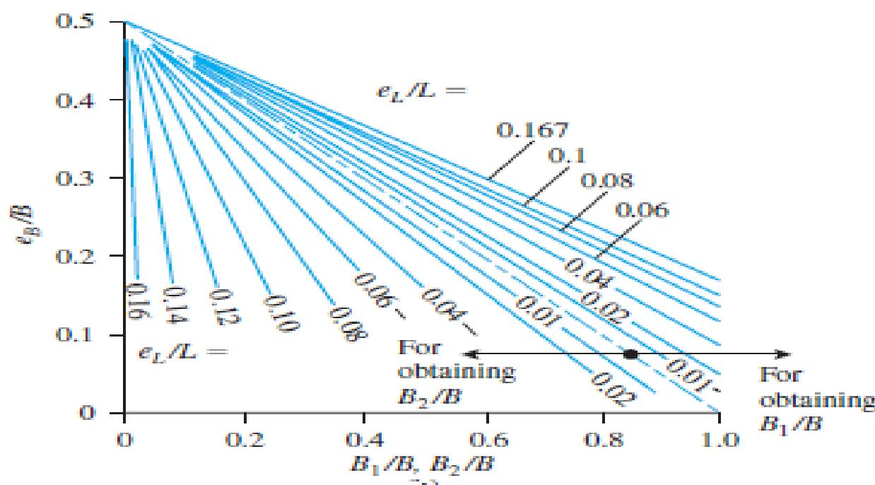
Effective area for the case of  $e_L/L < \frac{1}{6}$  and  $0 < e_B/B < 0.5$  (After Highter and Anders, 1985) Highter, W. H. and Anders, J. C. (1985). "Dimensioning Footings Subjected to Eccentric Loads," *Journal of Geotechnical Engineering*, American Society of Civil Engineers, Vol. 111, No. GT5, pp. 659–665. With permission from ASCE.)
