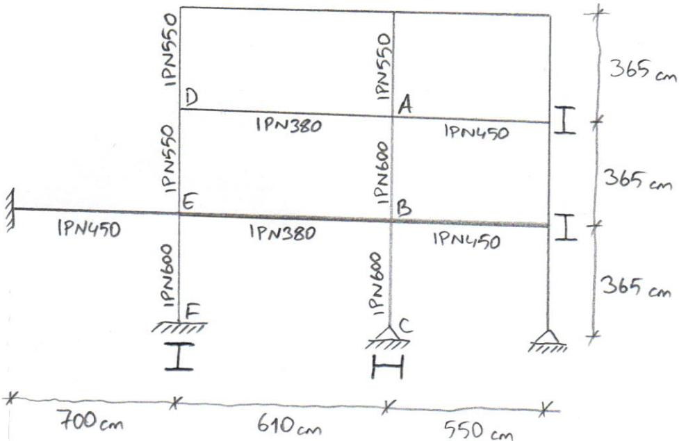
Determine effective length factors ( $K$ ) of AB, BC, DE and EF columns.
