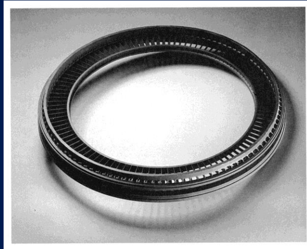
Figure 11 9 - A one-piece compressor stator with 108 separate airfoils made by investment casting (courtesy Howmet Corp )
