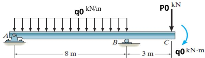
**Q3) Determine A and B support reactions.**
