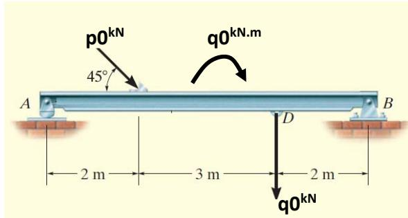
**Q2) Determine A and B support reactions.**
