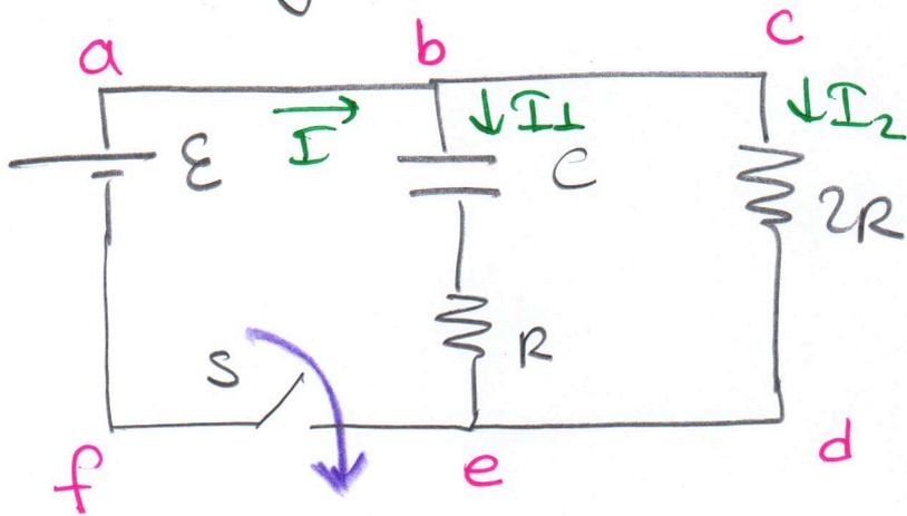
a) Find an expression for current  $I$  as a function of time and draw  $I=f(t)$  graphic when the capacitor is charging.
