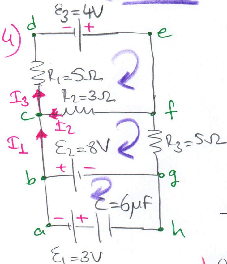
a) find the steady currents of  $I_1$ ,  $I_2$ , and  $I_3$  when the circuit is running for a long time.
