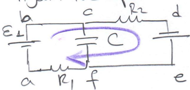
$$I = \frac{\mathcal{E}_1 + \mathcal{E}_2}{R_1 + R_2} = \frac{1 + 3}{0,2 + 0,3} = \underline{\underline{8A}}$$
