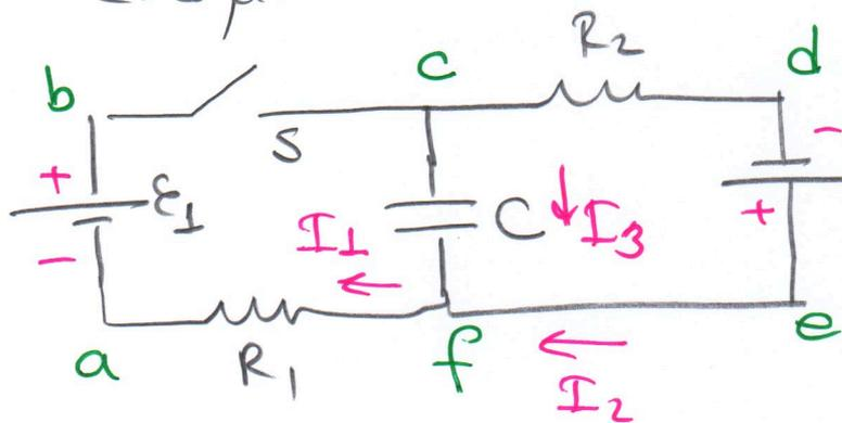
a) Find the currents in the circuit and the charge on the capacitor after a long time while S is still open.
