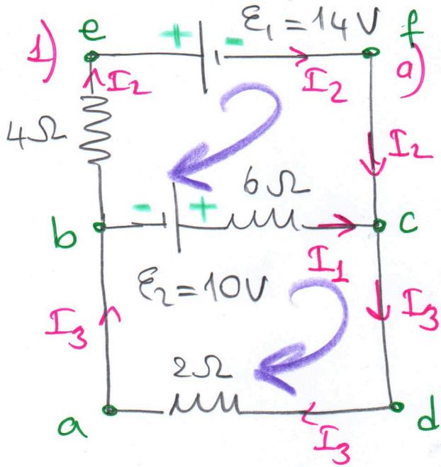
Find the currents  $I_1$ ,  $I_2$ , and  $I_3$  for the circuits
