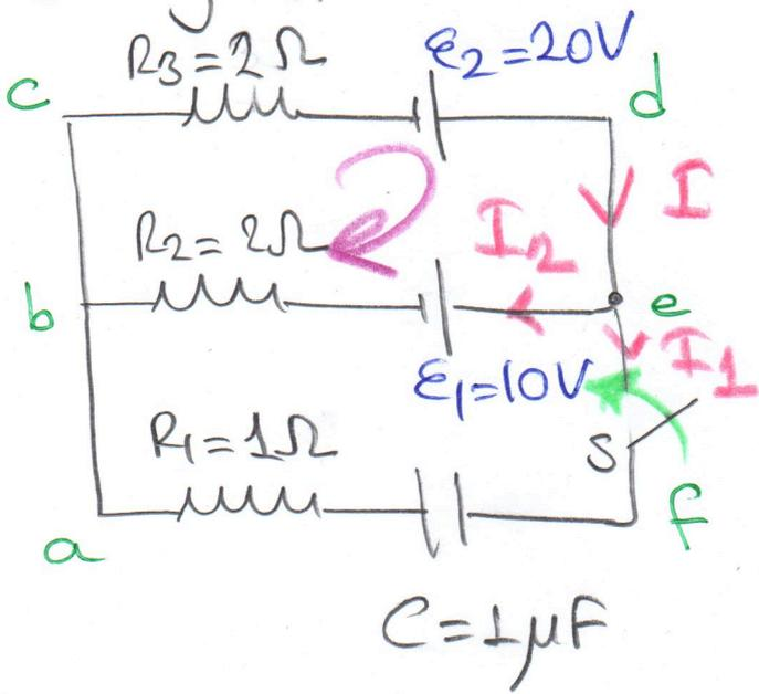
Steady state of the circuit corresponds to a fully charged capacitor. When the switch S is closed for a long time, the capacitor becomes fully charged and  $I_1 = 0$
