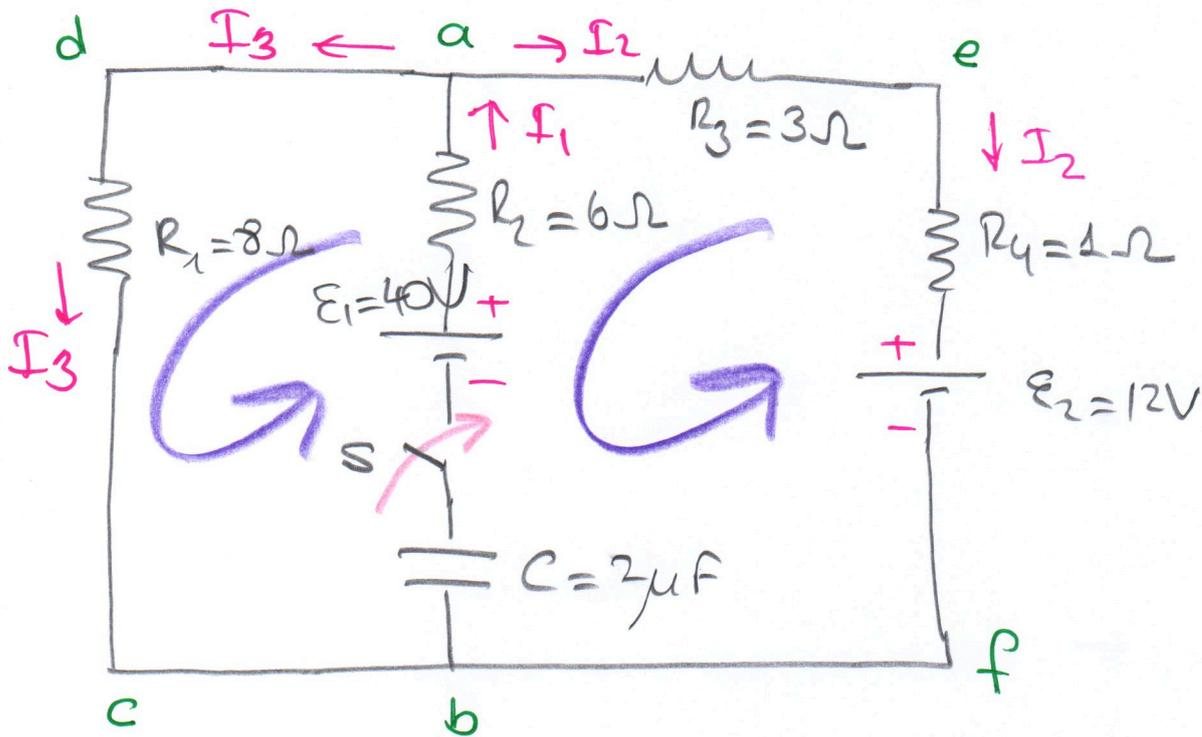
a) find the currents of  $I_1$ ,  $I_2$ , and  $I_3$  just after the switch S is closed.
